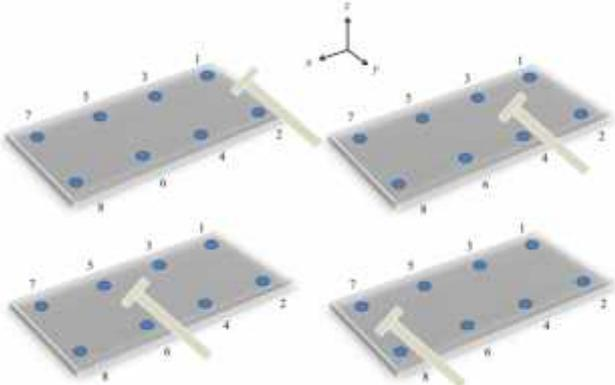
Figure 2: Roving hammer test
