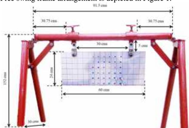
Figure 1: Fixed (Hinged) free steel plate
